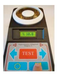
As soon as the "DISK"key has been activated the reading change (for 5 sec.) to read the average.
