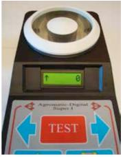
Continue to pour material into the measuring chamber until the display reads between 98 and 102 You will see that the lefthand arrow in the display changes to a horizontal arrow. If you pour too much in the chamber the arrow will point down - meaning too much in the chamber.
