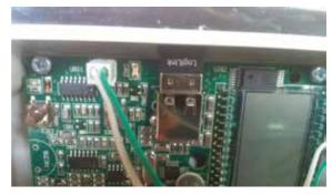
The connector with red/black wire must be mounted on the wireset with red/black wire comming from the pcb
