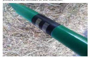
Tighten the fasteningnut. Do note that - as with ordinary spears - the spear can become loose by the every day use. Make sure to re-tighten the fasteningnut regulary to avoid damages to the spear & wire.
