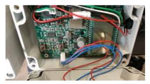
The lid is mounted and this concludes the mounting of spear & transmitter. Now connect the transmitters with the supply-cables.
