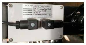
The head supply-cable (the cable connecting to the supply ) is mounted with a cigar-connector.
