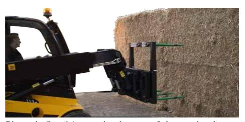
Telescopic handler with 6 spears and weighing-system. iPad is mounted in cabin. Bluetooth transfer between spears & weighing-system to iPad. No wires to cabin.
